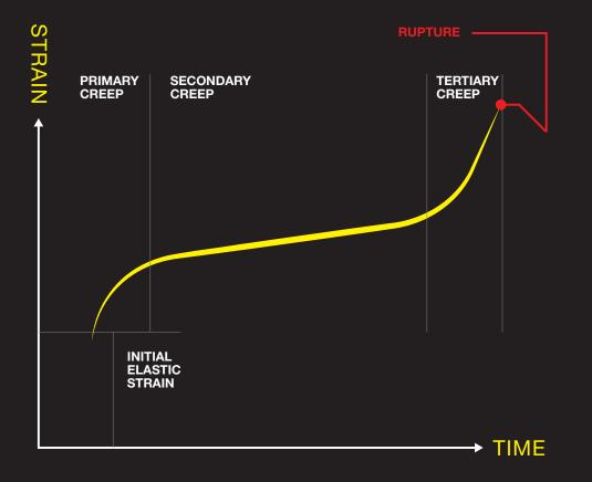
**Creep** is the tendency of a material to slowly deform over a long period exposed to stress (load or pressure), mostly below the yield strength, and elevated temperature.
