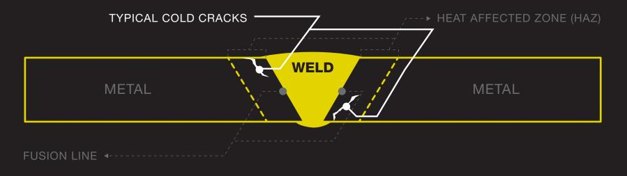
This is a type of cracking that appears after the welding (24-48hrs) and mainly at the HAZ (Heat Affected Zone). **AVOID:**
